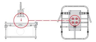
Place the truss mount on the rear side of the frame. Make sure that the 4 screws enter the 4 holes in the frame. Tighten the screws to secure the truss mount on the frame.
