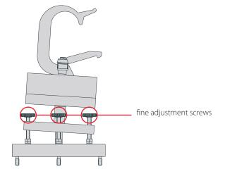
By means of the 4 adjustment screws, the positon of the truss mount can be defined very precisely.
