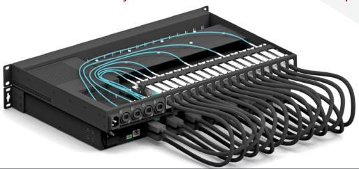
Combine an MX2-8x8-HDMI20-Audio matrix with a fully populated rack tray to create a Full 4K HDMI 2.0 optical matrix.
