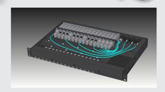
The PowerTray is a 1RU size housing accessory which can enclose up to 16 HDMI20-OPTJ-TX/RX90 units, also providing power source for every installed device. The optical fibers are connected to the four Neutrik OpticalCON Quad connectors, each carrying four signal fibers from four of the extenders. The HDMI tail cables of the extenders are accessible directly at the back of the PowerTray.
