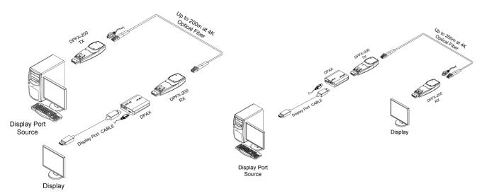
DPAX can improve transmission length of DPFX-200 via optical fiber. It has been confirmed that DisplayPort signal transmission length has improved up to 300m when using DPFX-200 with DPAX under certain environment such as below configuration. Each 200m and 300m of DisplayPort signal transmission has successfully tested when using GTX960 as a display source and ASUS PA328Q as a display.
